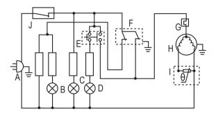
A-POWER PLUG C-GREEN LAMP E-QUICK FREEZING SWITCH F-THERMOSTAT G-OVERLOAD PROTECTOR H-COMPRESSOR I-PTC J-MAIN SWITCH
